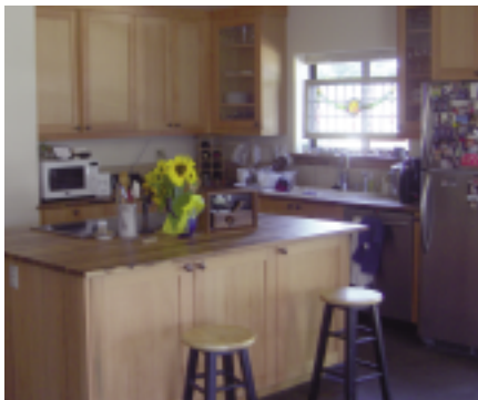
One goal of the Build Local Alliance is to promote the use of responsibly sourced wood from local vendors. FSC-certified lumber, urban trees, and salvaged wood from barrel staves were used to make the kitchen cabinets and countertops in this photo (courtesy of Bob and Julie Granger, Portland, Oregon).
